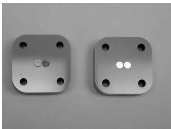
Fig. 1. Photograph of electrodes: Right: dual platinum electrode Left: dual glassy carbon electrode; the left side is the naked glassy carbon electrode, the right side is coated with the HRP enzyme.
